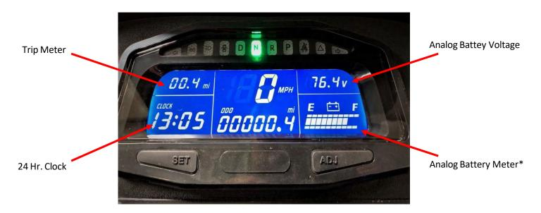
The dash display provides the vehicle driver with real time battery voltage conditions:
